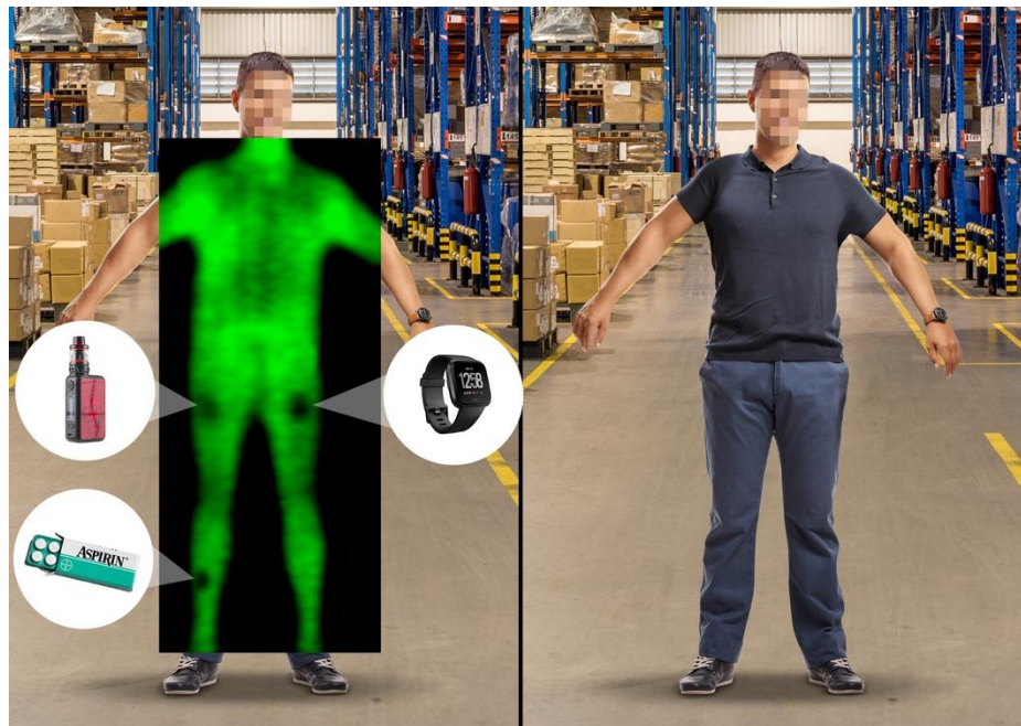
Thruvision’s unique passive terahertz technology allows a user to see the size, shape and location of stolen items concealed in clothing
