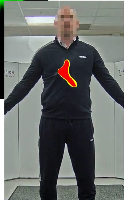
Thruvision’s AI-based Dynamic Detection algorithm shows gun as alarm overlay
